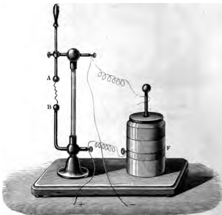
FIG. 71.—Figure showing how the jar is connected with the spark stand. A, B, poles; F, jar
